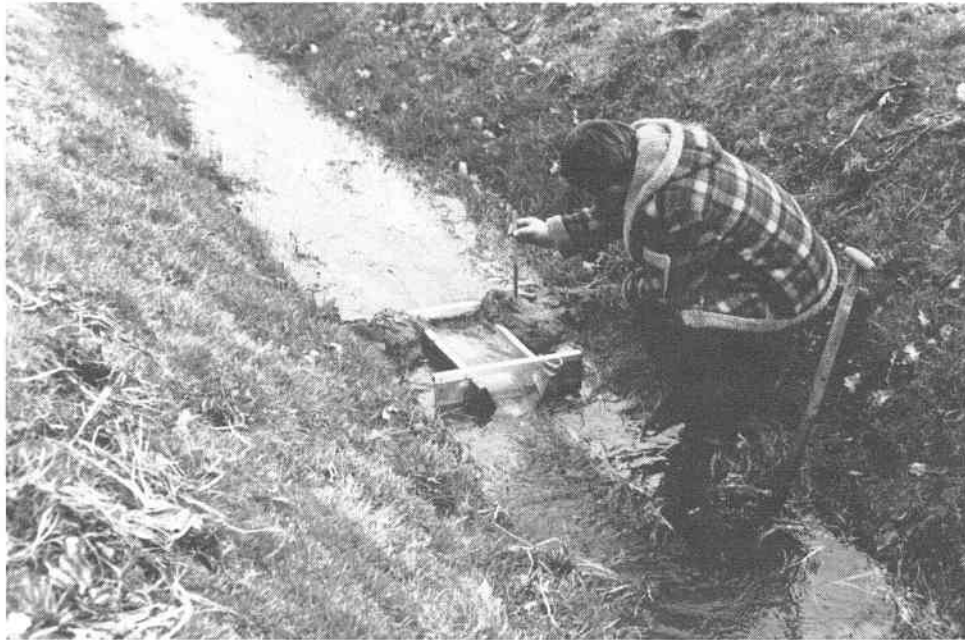
Photo 1 Long-throated flumes can be portable
