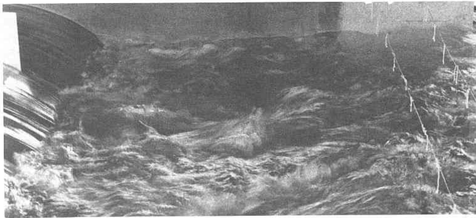
Design B Tailwater depth is 15% greater than in Design A
